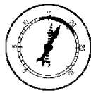
POOR VALVE SEATING AT IDLE
